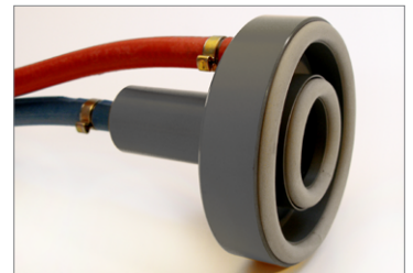
Two-chamber vacuum cell with sealing rings
